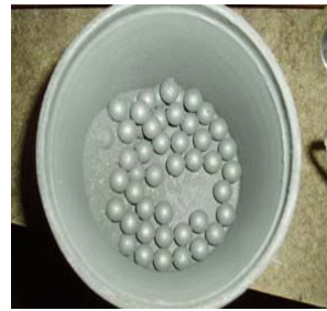
Figure 5-b An example of Grinding media for ball mill (Lead antimony-grinding media with aluminum powder)
